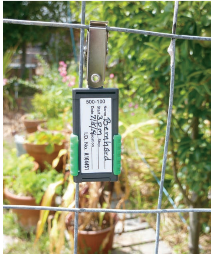
Formaldehyde badge clipped to an outdoor fence; a common air monitoring technique.
