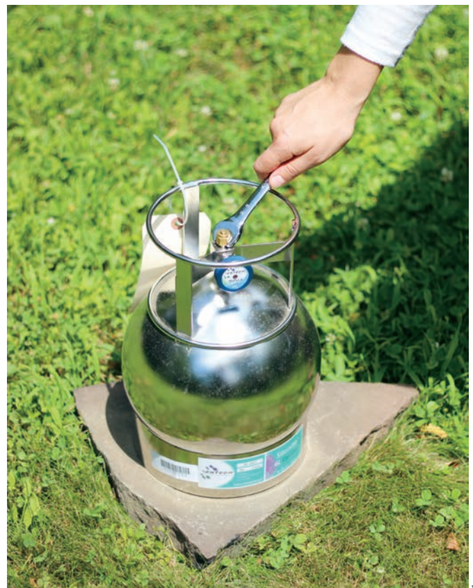
Summa canisters are frequently used by government agencies and communities to take air samples.
